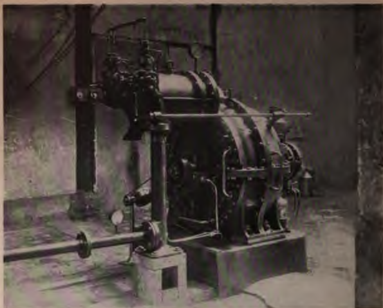
FIG. 84.—The Armengaud and Lemale gas turbine. This view shows the combustion chamber, air and fuel inlets and connections.
